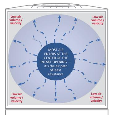
The further away you get from the center of the tower, the lower the air volume and velocity entering the cooling tower fill; upper and lower corners have the lowest air volume and velocity entering the fill.
